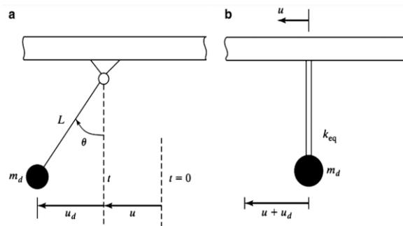
[Fig. 1]: A simple pendulum TMD and Equivalent system (Connor & Laflamme, 2014)
