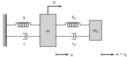
[Fig. 2]: Single Degree of Freedom - TMD system
