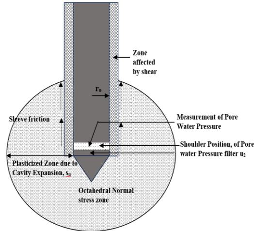
Figure 1: Stresses along with cavity expansion zone during cone penetration
