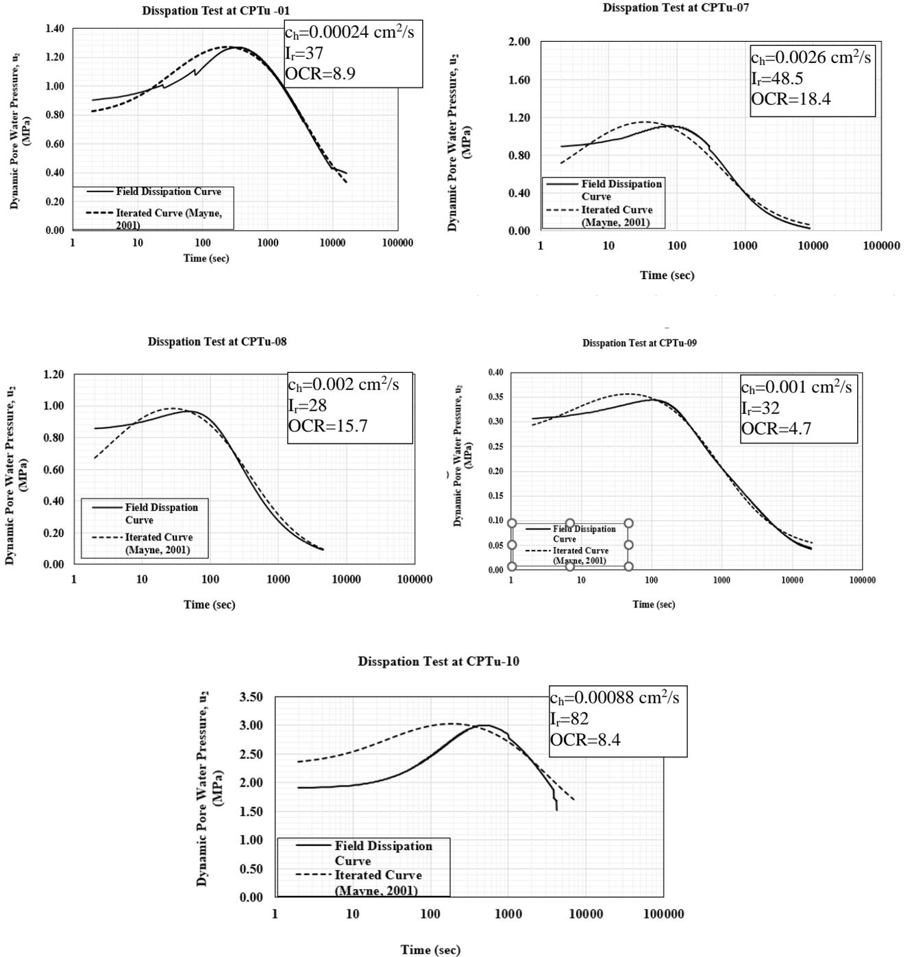
Figure 7: Determination of  $c_h$  using iteration method by Mayne (2001) for dilatatory Curve at CPTu-01, CPTu-07, CPTu-08, CPTu-09 and CPTu-10
