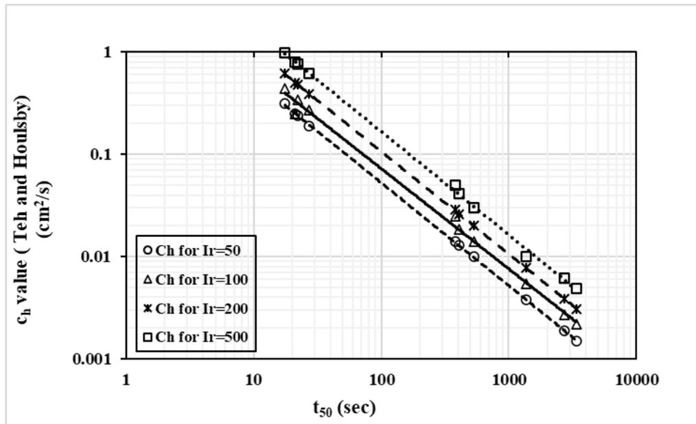
Figure 5:  $t_{50}$  vs  $c_h$  plot for Rigidity Index,  $I_r=50$  to 500 using Teh & Houlsby (1991) method
