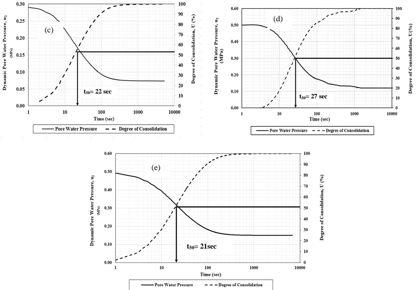
Figure 3: Determination of  $t_{50}$  from monotonic curve for (a) CPTu -02, (b) CPTu -03, (c) CPTu-04
