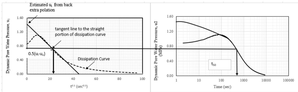
Figure 2: Estimation of  $t_{50}$  for dilatory curves using Square root of time proposed by Sully et al., (1999)
