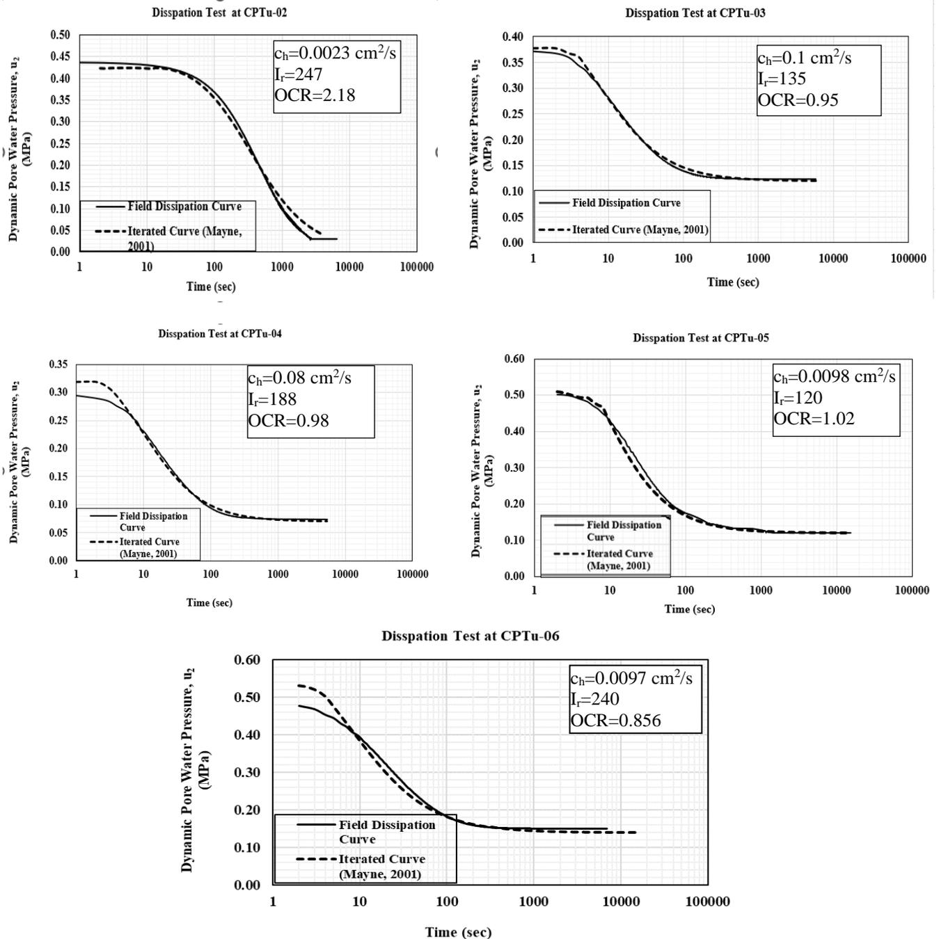
Figure 6: Determination of  $c_h$  using iteration method by Mayne (2001) for monotonic Curve at CPTu-02, CPTu-03, CPTu-04, CPTu-05 and CPTu-06
