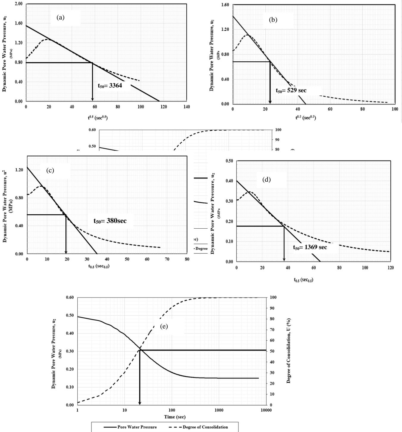
Figure 4: Determination of  $t_{50}$  from dilatory curves using Sully et al. (1991) method for (a) CPTu-01, (b) CPTu-07, (c) CPTu-08, (d) CPTu-09 and (e) CPTu-10
