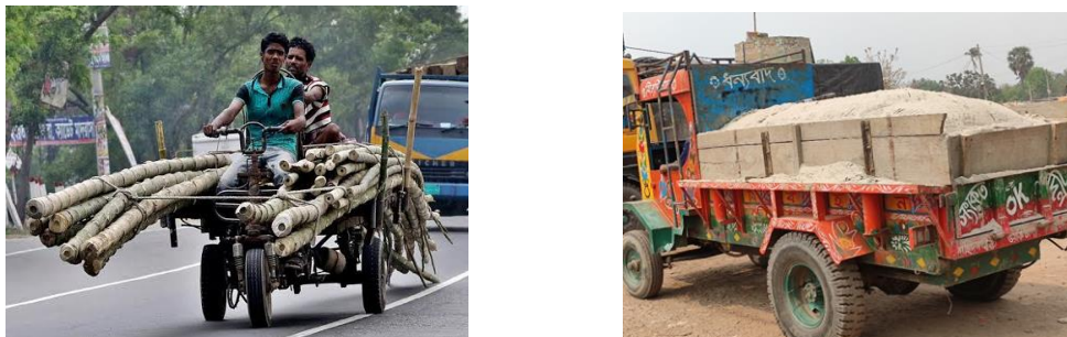
Figure 1: Three-wheeler and four-wheeler SEV for carrying comparatively lightweight and heavy weight load
