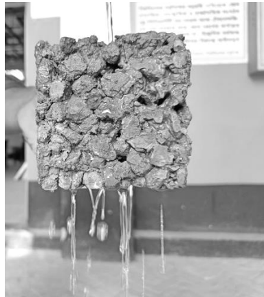
Figure 1: Highly porous concrete
