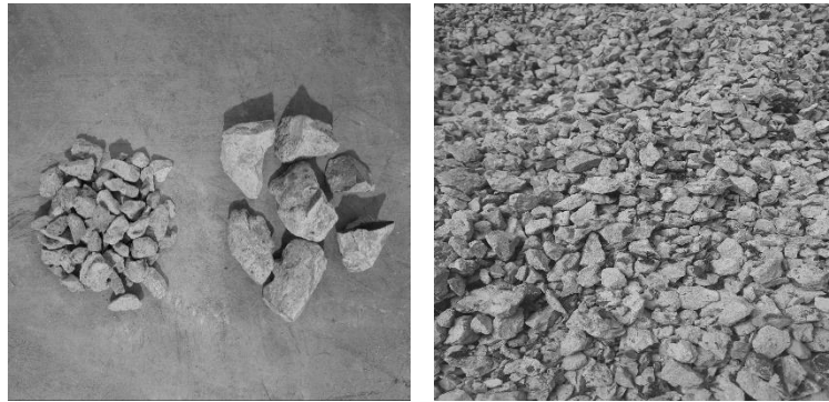
Figure 1: 10-20mm and 10-12mm RCA from demolished pile head.
