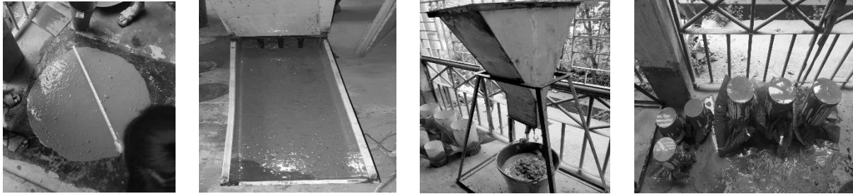
Figure 5: Workability tests and casting of SCC.
