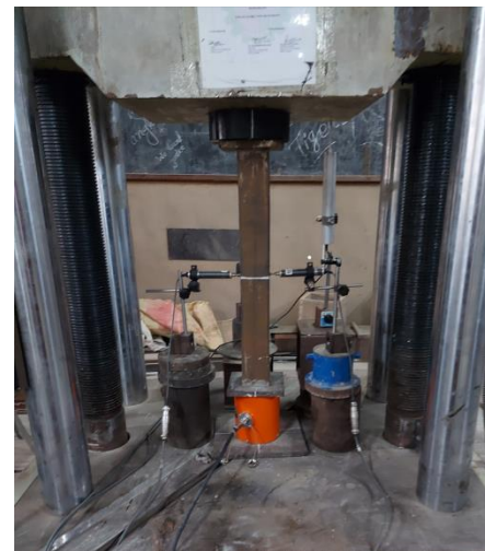
Figure 3: Test setup and instrumentation for CFST columns in laboratory
