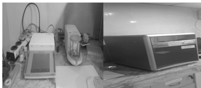
Figure 3: Experimental apparatus for elemental analysis of MSW (Vario Micro Cube Elementary)
