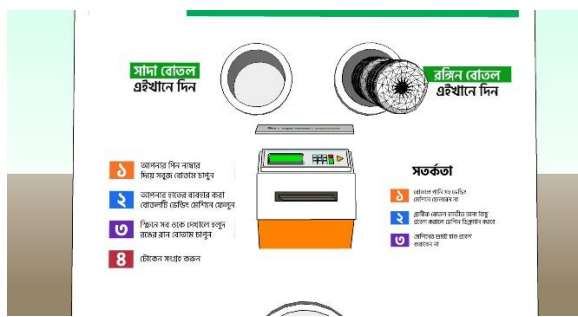
Figure 13: ProCritic RVM with separate input holes for coloured and white bottles
