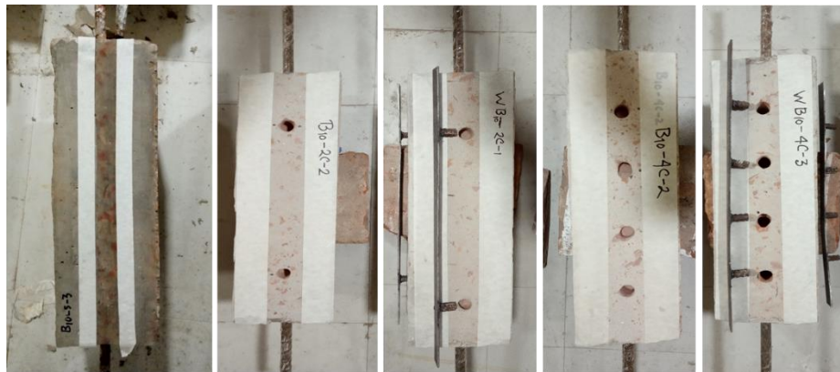
Figure 2: Strengthening of prism specimens.
