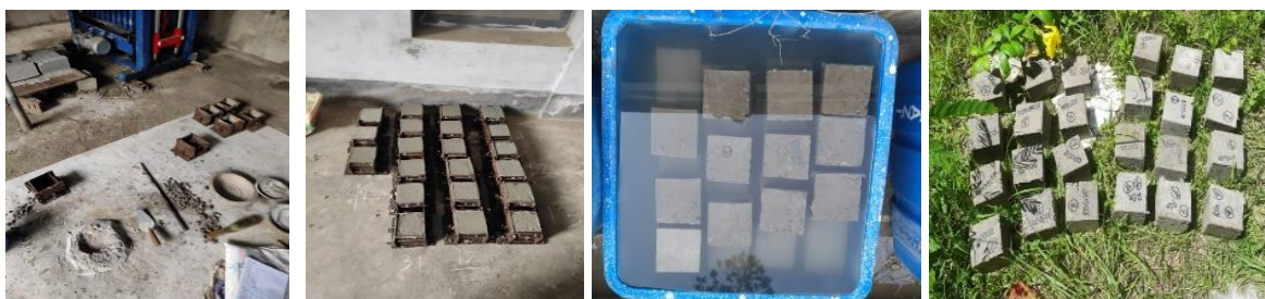
Figure 3: Mixing, Molding, Curing, and Preparation of Specimens for test
