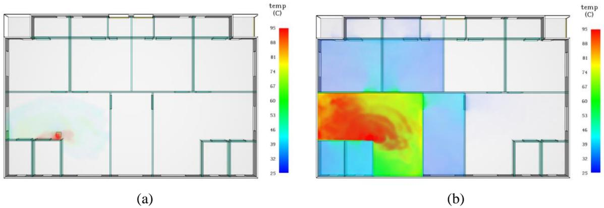
Figure 4. Fire growth timeline in PyroSim.
