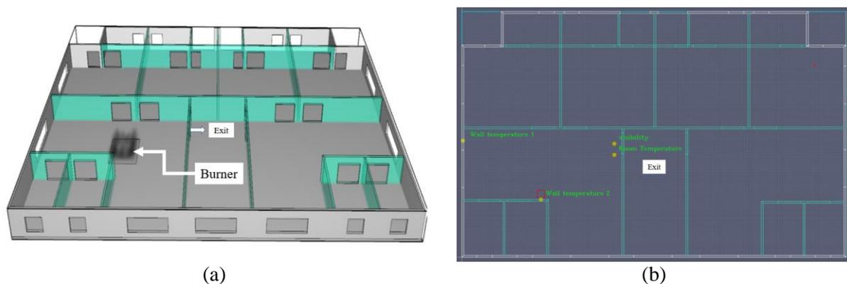
Figure 3: (a) Fire source; (b) Device location.
