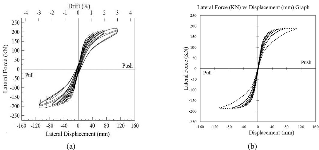
Figure 5: Comparison of force displacement response; a) Experimental, b) Numerical
