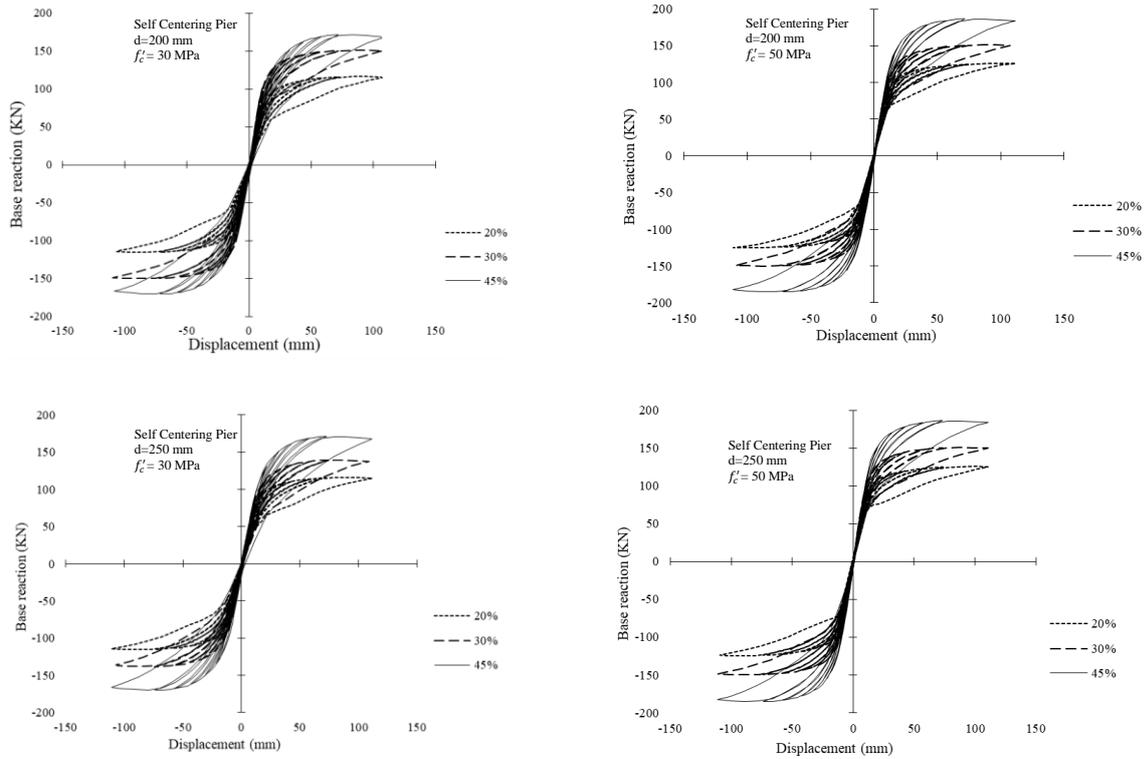
Figure 6: Base Reaction vs Displacement
