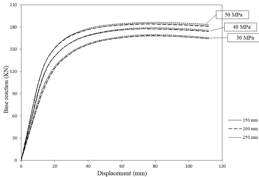
Figure 7: Base Reaction vs Displacement graph for variable duct diameter.
