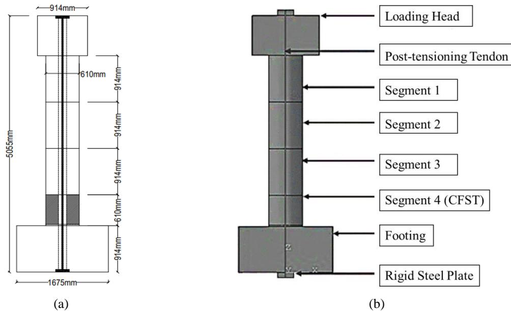
Figure 1: (a) Geometry, (b) FE Model
