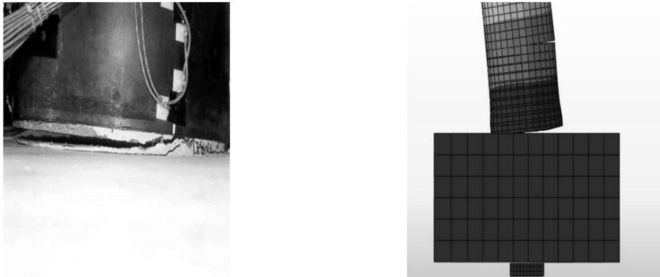
Figure 4: Separation between foundation and CFST section
