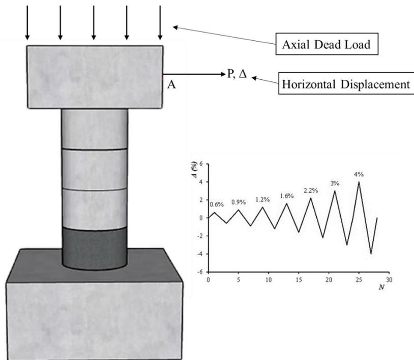
Figure 2: Schematic diagram of the bridge pier loading
