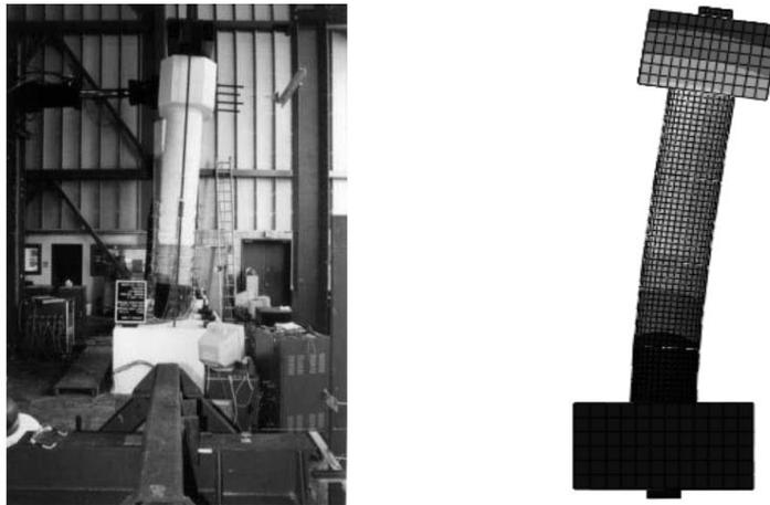
Figure 3: Comparison between deformed shape
