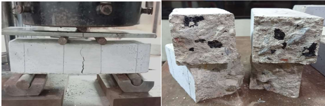
Figure 6: Test setup to determine flexural strength of concrete and failure surface of recycled aggregate that contains EAFS.
