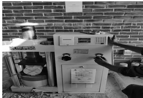
Figure 5: Application of load to the cylindrical specimen to determine the split tensile strength
