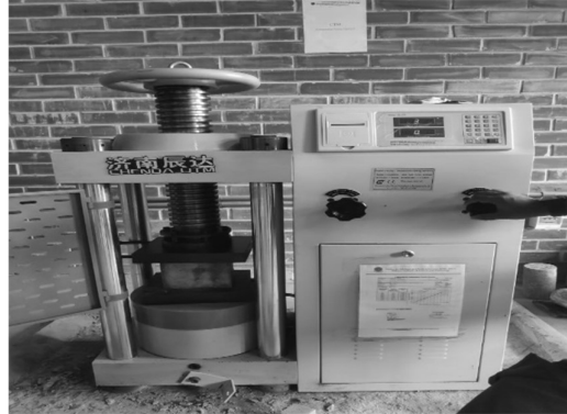
Figure 4: Application of load to the cube specimen to determine the compressive strength
