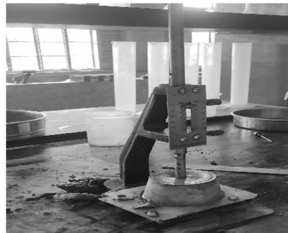
Figure 7: Determination of standard consistency of cement paste with the help of Vicat's Apparatus
