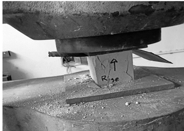
Figure 2: Compression test of AAC cube units.
