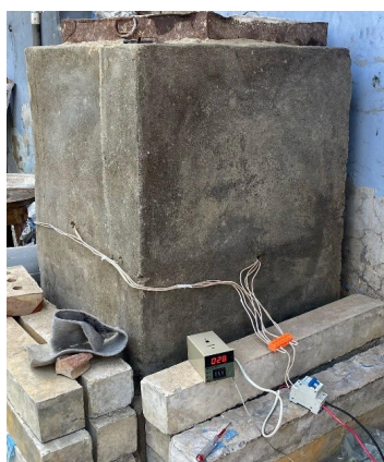
Figure: 3.1.1 Burning of column at burn chamber
