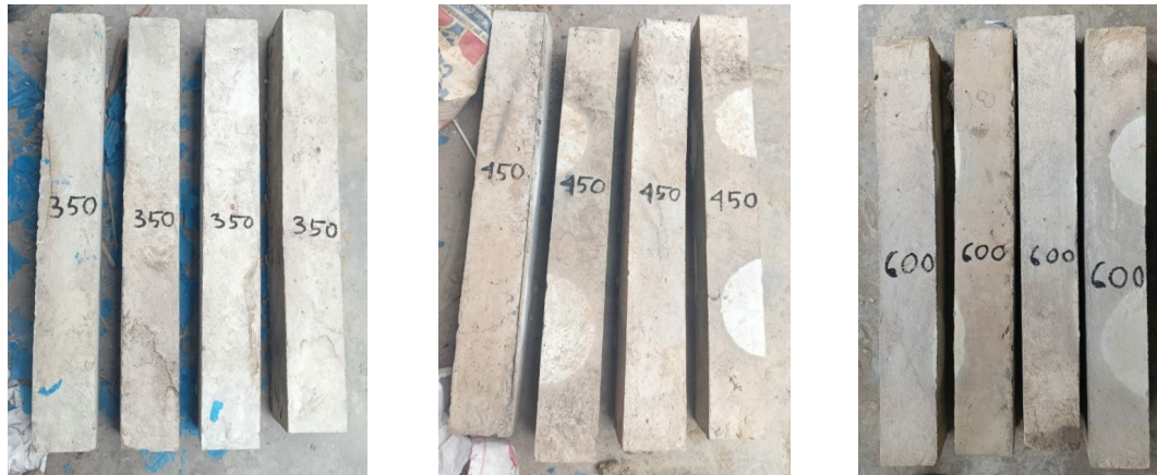
Figure 3.1 Columns after fire damage at 350, 450 & 600 degree centigrade respectively
