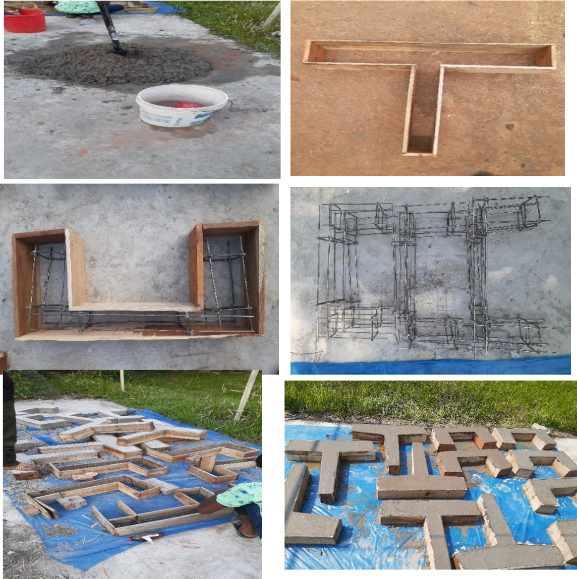
Figure 3: Concrete mixing, T & C wooden forma, column reinforcement and casted different type of specimens
