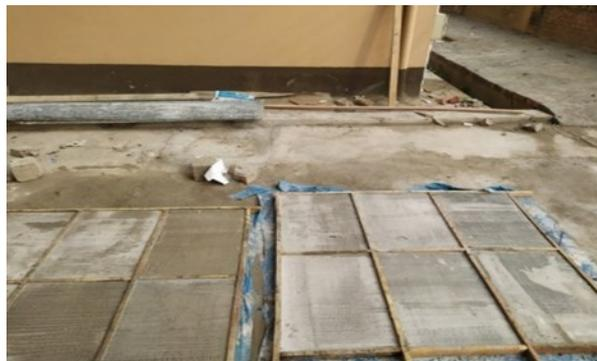
Type A: 1.25% reinforcement (Mesh opening-12.5 mm).
