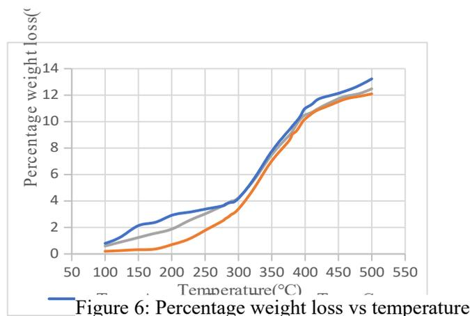
Figure 6: Percentage weight loss vs temperature
