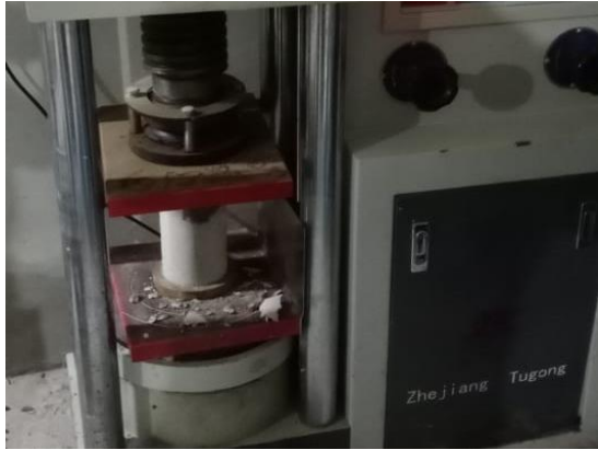
Figure 4: Compressive strength test according ASTM C39
