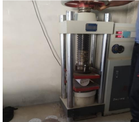
Figure 5: Split tensile strength test according ASTM C496
