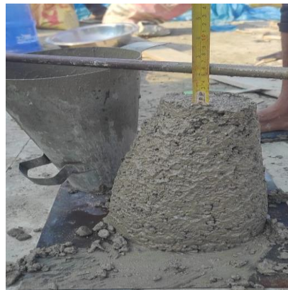
Figure.3: Measure workability of concrete according ASTM C143
