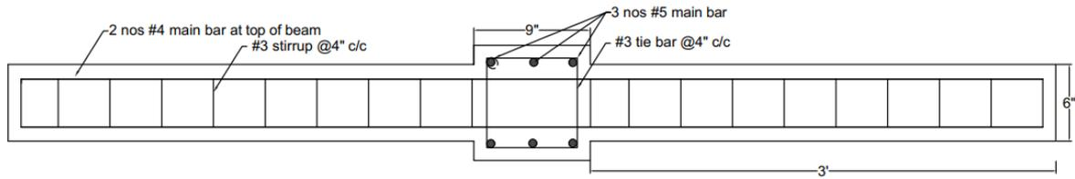
Figure 3: Reinforcement Detailing of Beam column joint (top view).
