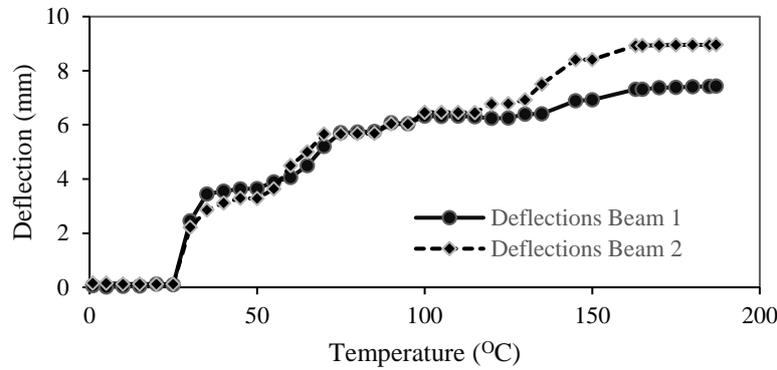
Figure 10: Variation of deflection with time due to exposed high temperature
