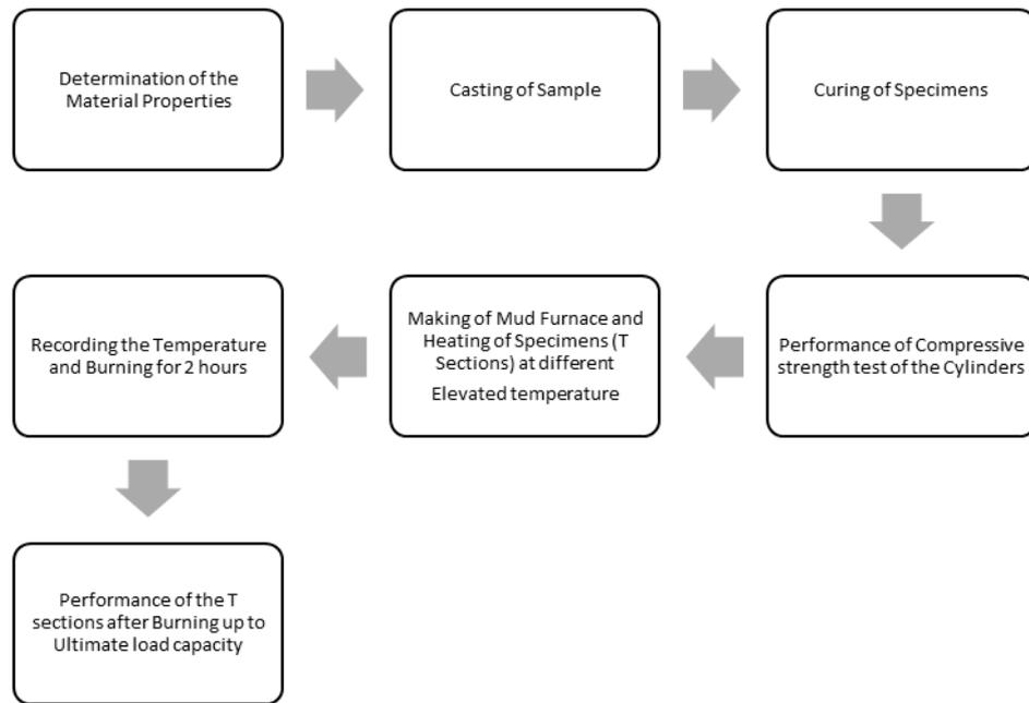
Figure 1: Flow diagram of the experimental process
