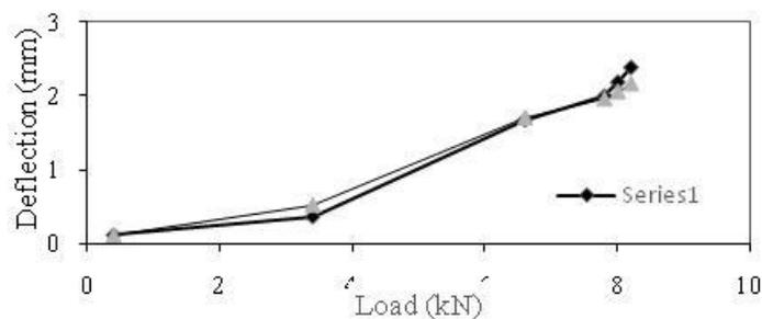
Figure 5: Deflection of Beam at working load
