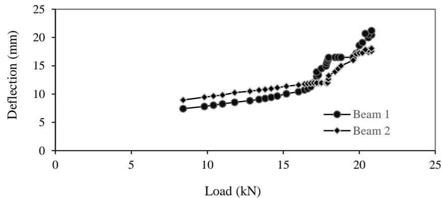
Figure 32: Variation of deflection of beam loading
