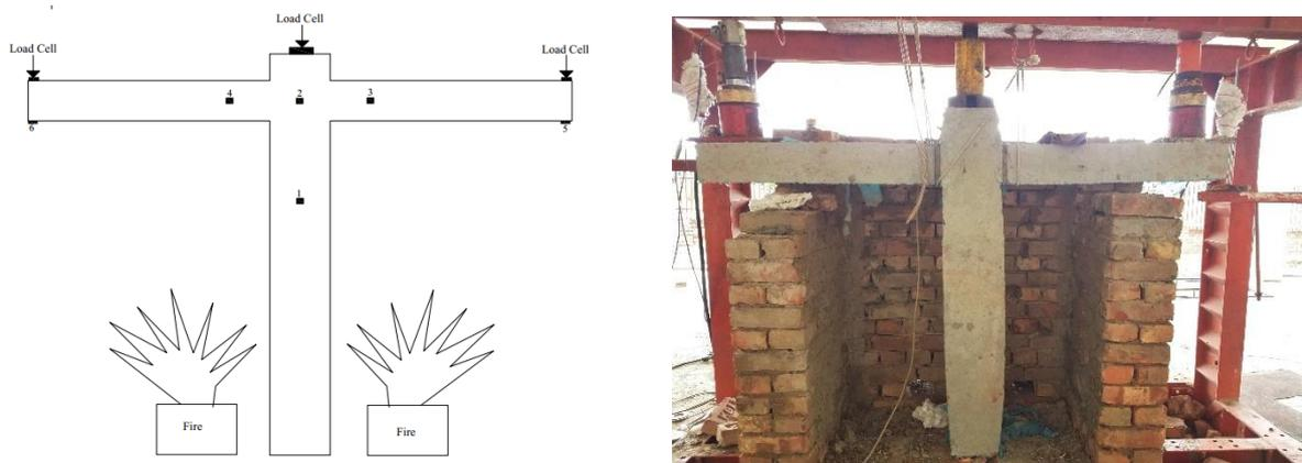
Figure 4: Mud furnace and load setup for experiment
