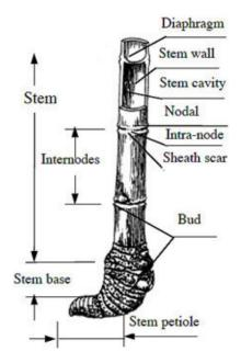
Figure 1: Schematic of bamboo stem (Guadua Bamboo, 2023b)
