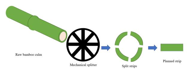
Figure 4: Steps to obtain planned strip for engineered bamboo production
