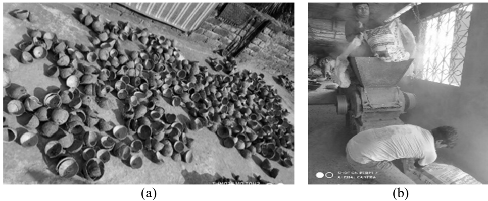
Figure 2: Coconut Shell Aggregate (a) collection of raw coconut shell; (b) grinding of coconut shell
