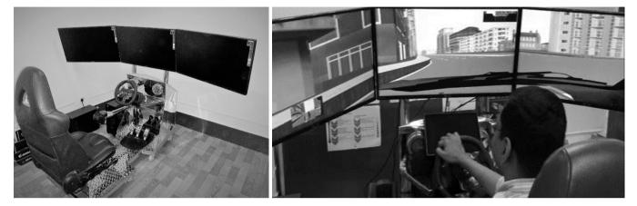
Figure 1: a) The driving simulator platform at BUET (left); b) The Experimental driving simulator with a predefined driving environment (right).
