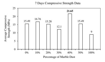
Figure 4 : Bar diagram showing the variation in strength for 7 days test
