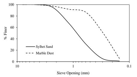
Figure 2: Gradation curve for sylhet sand and marble dust
