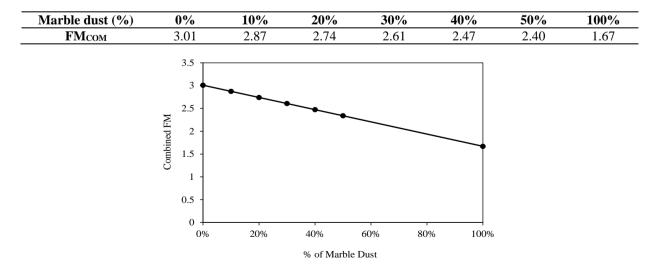
Figure 3: Combined fineness modulus of fine aggregate
