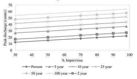
Figure 6: Variation of discharge with % impervious in different return periods
