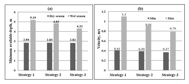
Figure 8(a): Minimum available navigation depth (b) Maximum and minimum velocity for the three proposed dredging strategies
