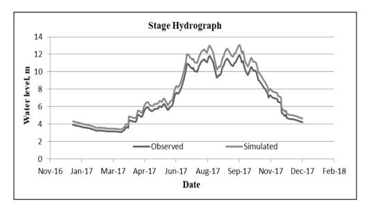
Figure 3: Validation of water level at Tilli of Dhaleswari River
