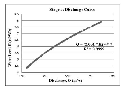
Figure 6: Rating curve using conveyance analysis
