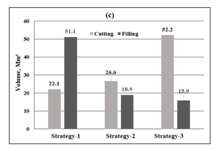
Figure 8(c): Cutting and filling volume for the three proposed dredging strategies
