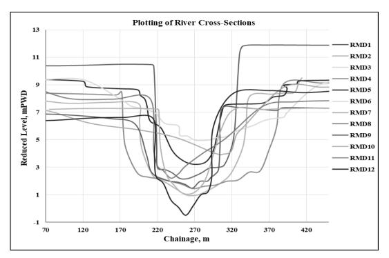
Figure 4: Plotting of original bathymetry
