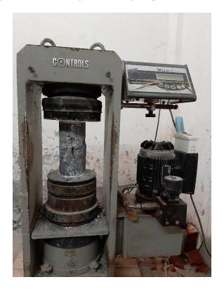
Figure 3: (a) Compressive strength test, (b) Tensile strength test
