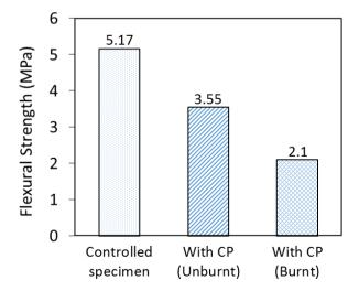
Figure 3: Comparison of flexural strength of beam specimens
