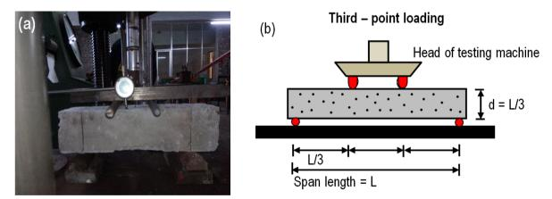
Figure 2: Flexure Test of Concrete by third-point loading method; (a) Photograph of test setup, (b) Schemetic view of test setup.
