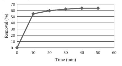
Figure 2: Effect of time on adsorption of methylene blue
