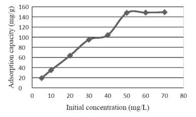
Figure 4: Effect of initial concentration on adsorption capacity
