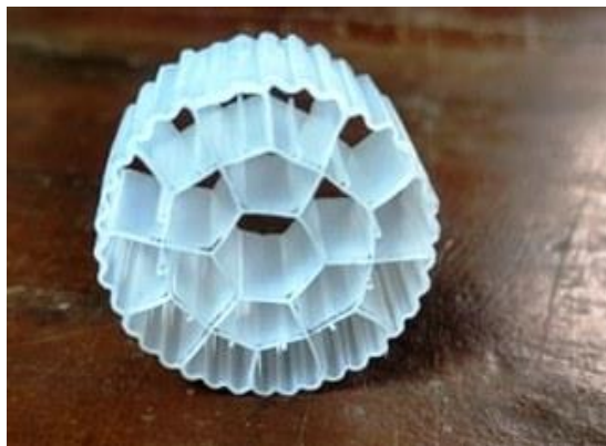
Figure 9: (a) kaldnes K3 media before using in experiment (b) kaldnes K3 media after ending the experiment with biomass
