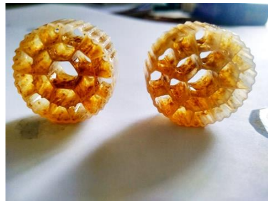
Figure 9: (a) kaldnes K3 media before using in experiment (b) kaldnes K3 media after ending the experiment with biomass
