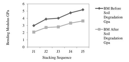
Figure 9: Reduction of Tensile Modulus for Soil degradation
