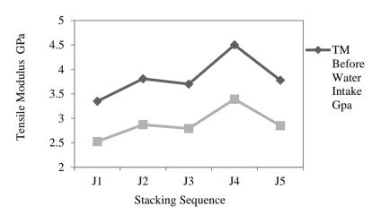
Figure 8: Reduction of Tensile Modulus for Soil degradation
