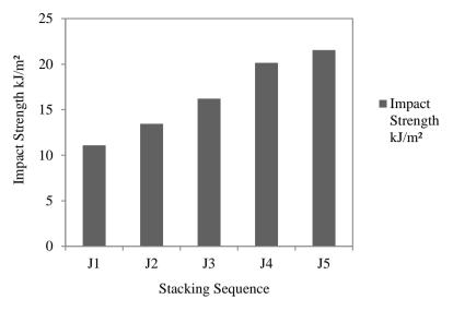
Figure 4: Impact strength with increasing stacking sequence
