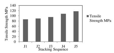
Figure 1: Variation of tensile strength with stacking sequence
