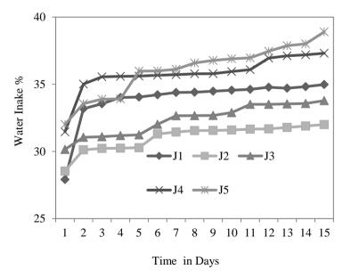
Figure 5 : Water intake increase with stacking sequence
