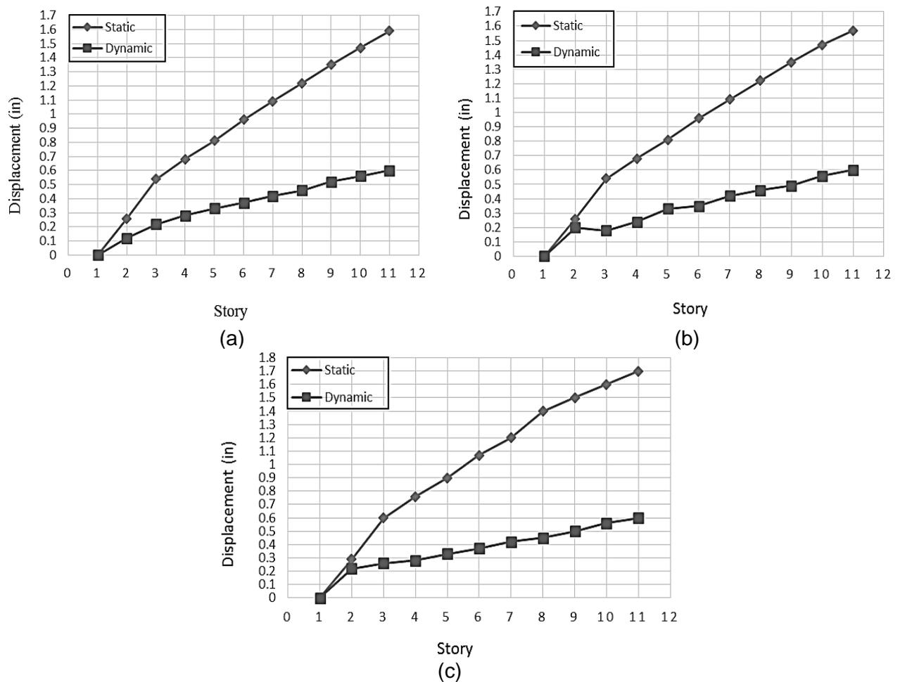
Figure 5: Comparison of displacement Profile under static and dynamic loading at (a) corner column (b) external middle column (c) central column.
