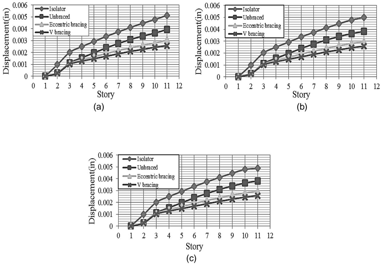
Figure 3: Displacement Profiles under Fukushima earthquake at (a) corner column (b) external middle column (c) central column.
