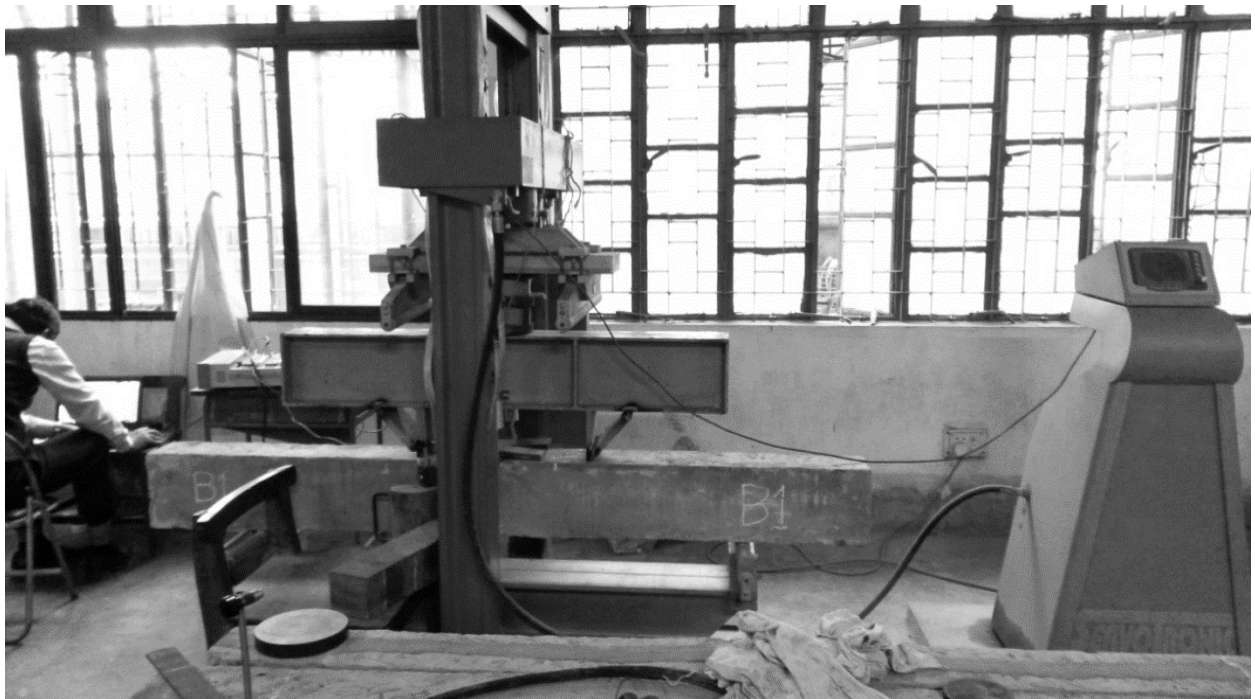
Figure 3: Typical loading arrangement
