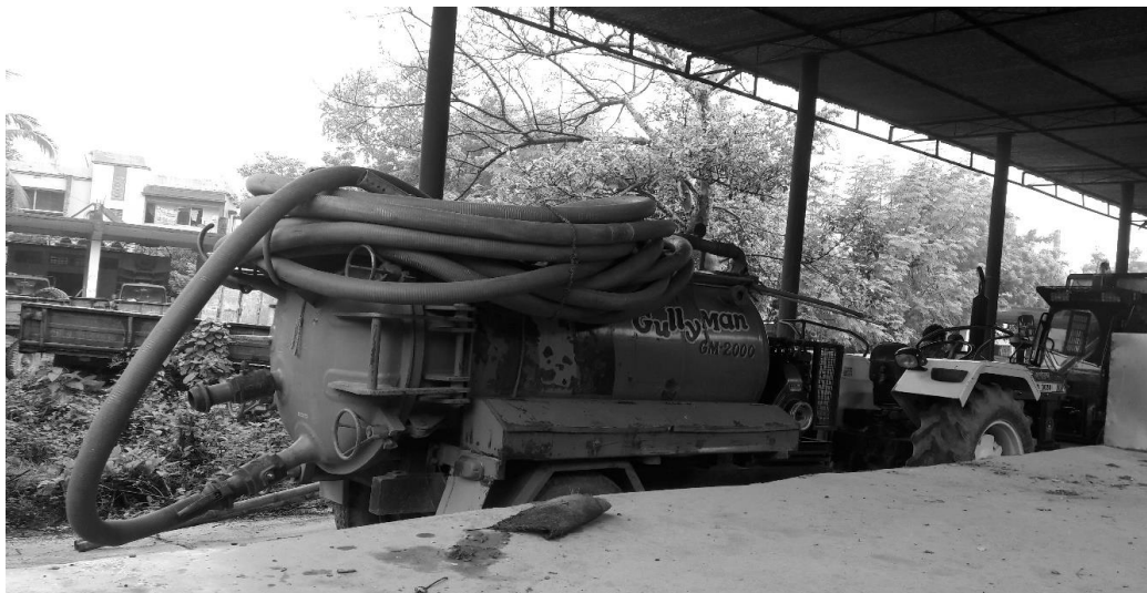
Figure 2: Desludging Vacuum Tanker with Tractor
