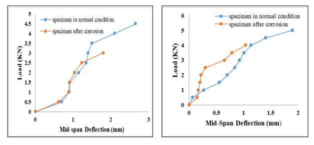
Figure 6: Load and deflection for specimen A
