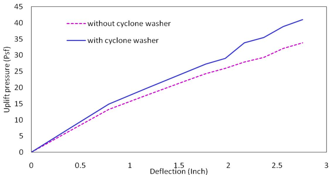
Figure 15: Comparison the effect of cyclone washer at mid point of the specimen
