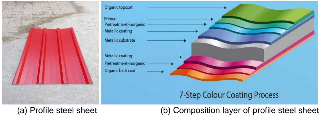
Figure 3: Profile steel sheet and its composition
