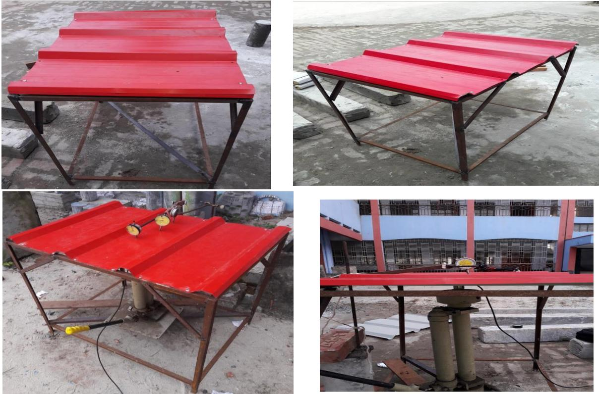
Figure: 12 Test arrangement of wind uplift load
