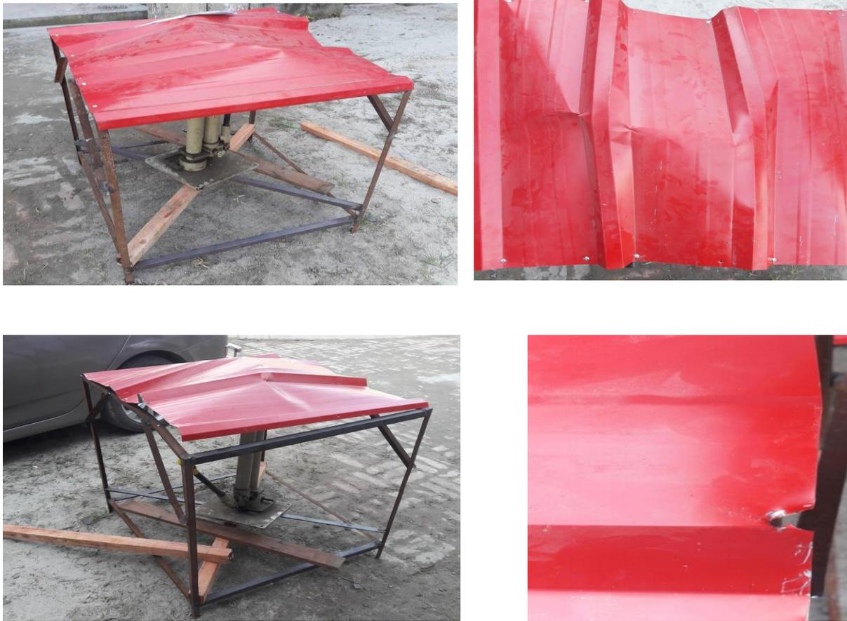
Figure 13: Failure mode of uplift pressure
