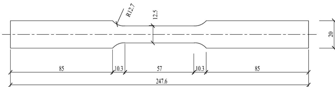
Figure 4: Dimension (mm) of coupon test specimen
