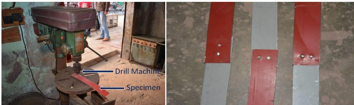
Figure 7: Drilling and conneting of tensile test specimen
