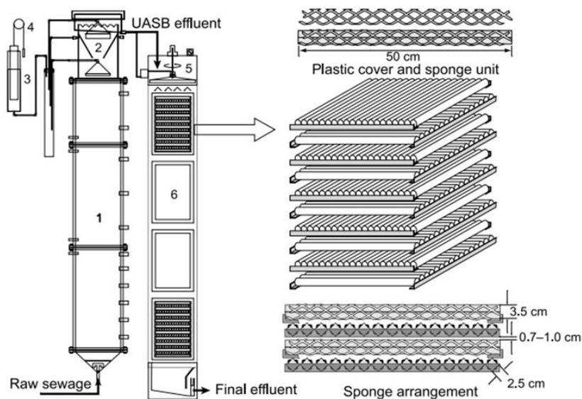
Figure 1: UASB bioreactor combined with DHS reactor
