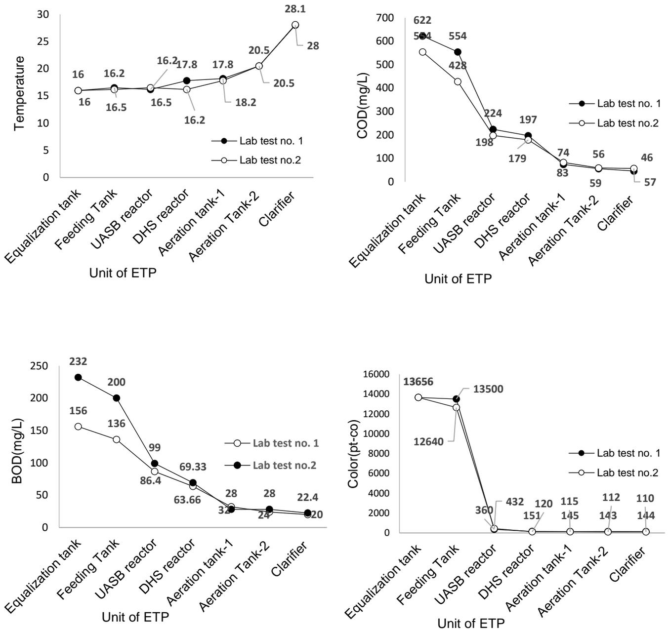
Figure 3: Dissolved oxygen, pH, turbidity, electric conductivity, temperature, chemical oxygen demand, biological oxygen demand and color profile of UASB combined with DHS treatment process for two laboratory test.
