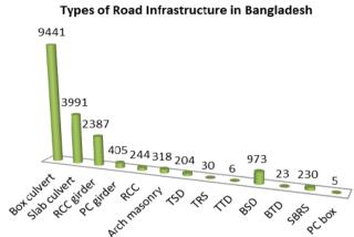
[Here, TSD = Truss with Steel Deck, TRS = Truss with RCC Slab, TTD = Truss with Timber Deck, BSD = Baily with Steel Deck, BTD = Baily with Timber Deck, SBRS = Steel Beam and RCC Slab, PC = Pre-stressed concrete]
