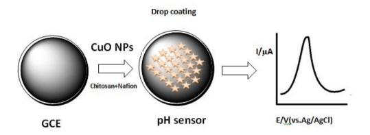
Figure 2: Schematic diagram on fabrication of pH sensor.
