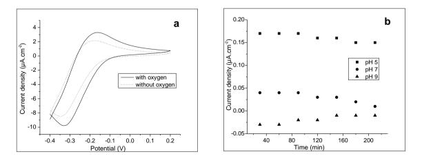
Figure 4: (a) CVs showing the response of the CuO immobilized layer to the presence and absence of oxygen in pH 6 buffer; (b) Electrode drift of CuO immobilized on the GCE; potential readings of pH 5, 7 and 9, signals have been taken every 30 min over a period of 3 hours.
