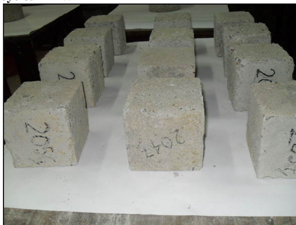
Plate No.4: FA Concrete specimens after 90 F-T cycles in PW
