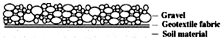
Figure 4:Illustration of a geotextile fabric separating a gravel layer from the underlying soil material. (~ Ohio line/aex-fact/0304.html )
