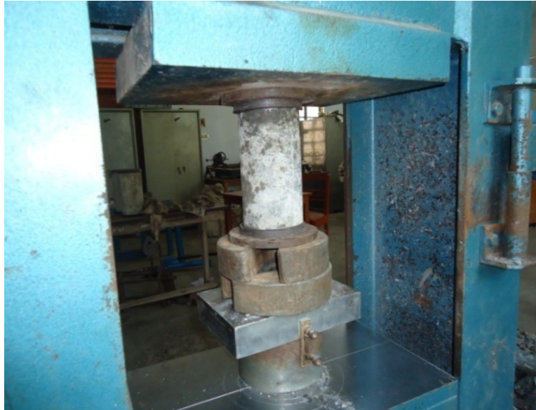
Figure 8: Compressive strength test of pervious concrete
