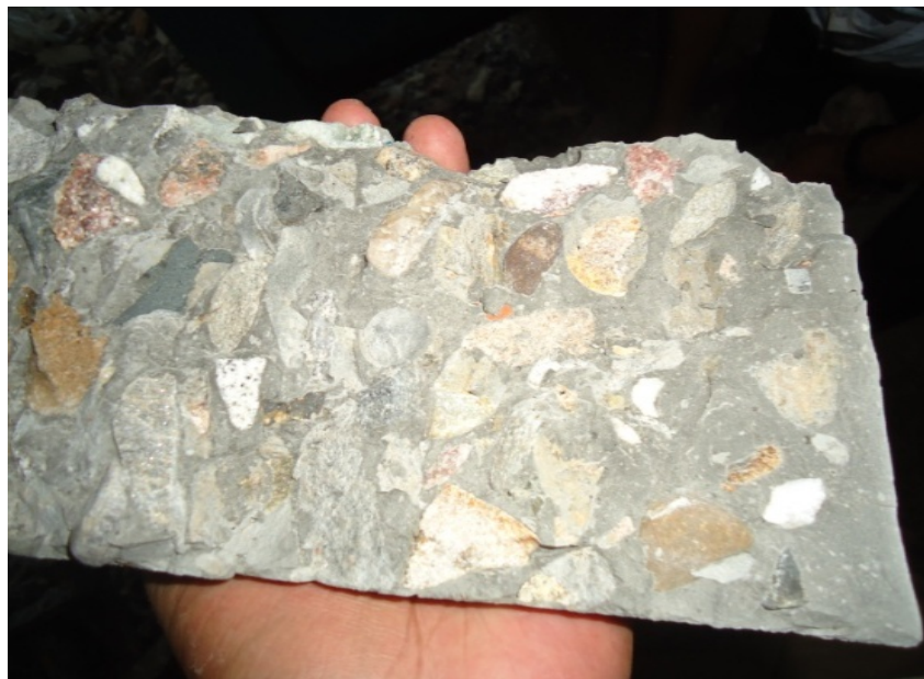
Figure 11: Failure behaviour of split tensile strength test of pervious concrete
