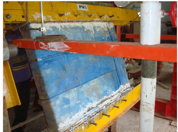
Figure 13. Out-of-plane movement of wall PW1
