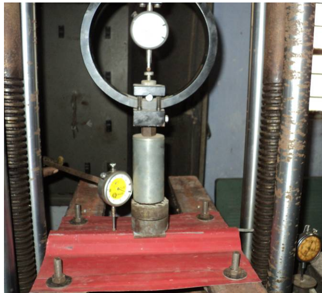
Figure 11: Test setup of web crippling test
