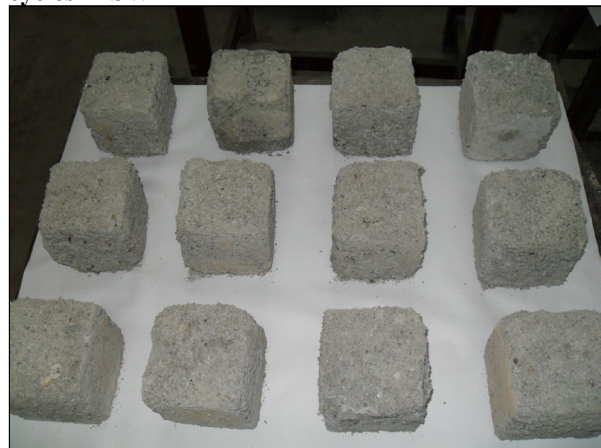
Plate No.4: FA Concrete specimens after 90 F-T cycles in SW
