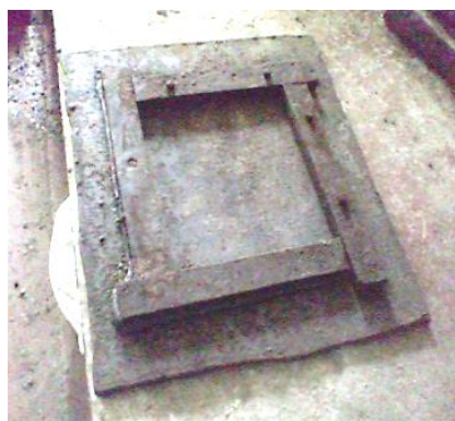
Figure 19: Mold for sulfur capping
