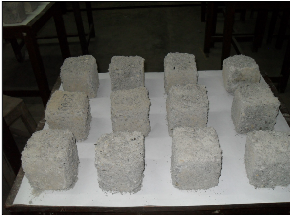
Plate No.6: FA Concrete specimens after 180 F-T cycles in PW
