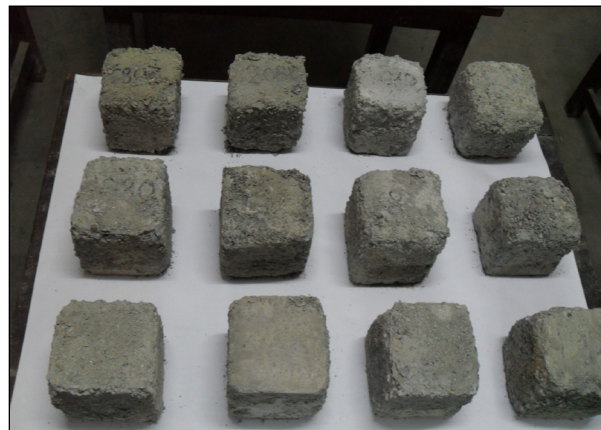
Plate No.3: FA Concrete specimens after 30 F-T cycles in SW
