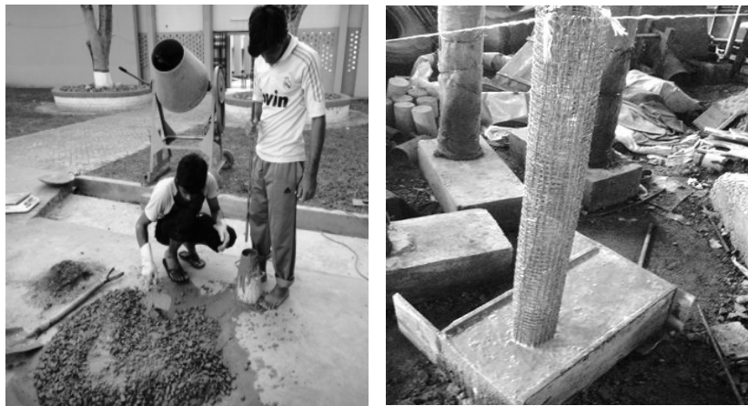
Figure 5: Casting of the column specimens
