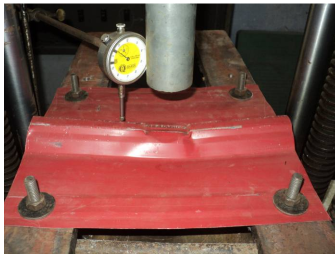
Figure 12: Failure of mode of web crippling test specimen
