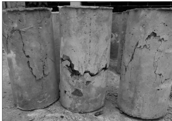
Figure 2: Compressive strength test (Universal testing machine).
