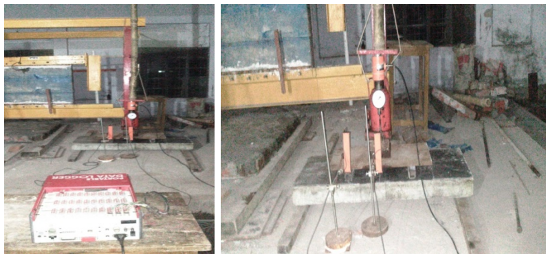
Figure 10: Laboratory Test set up of Slab Specimens
