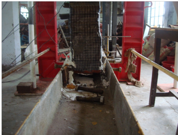
Figure 12. Premature failure of CW1 due to slip of anchorage at wall bottom.
