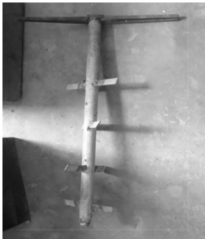
Figure 6: Mixing Device for Installation of Cement Column
