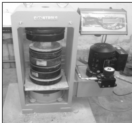
Figure 5: Compressive Strength Test of Mortar
