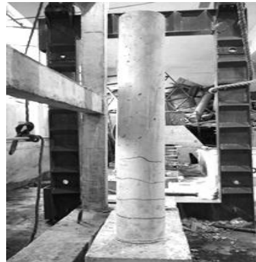
Figure 9: Cracks in Ferrocement Column
