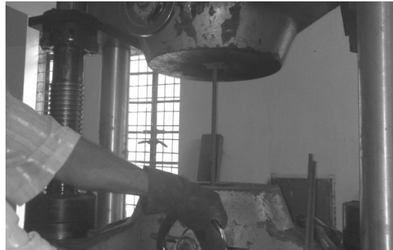
Figure 2: Test Set up for yield strength test of reinforcement
