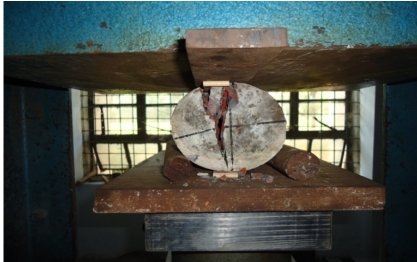
Figure 10: Split-Tensile Strength test of pervious concrete
