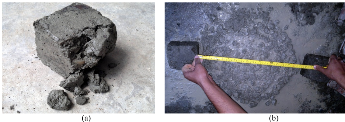
Figure 2: (a) Effect of admixture for high dosing, and (b) Slump Flow diameter
