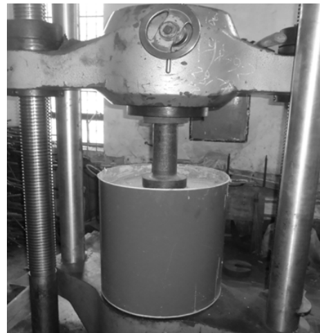
Figure 7: Load Settlement Measurement
