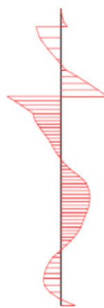
Figure 9: Shear force in (Max SF=75kN/m) and Forces in the top and bottom ties are 83 kN/m and 240 kN/m, respectively.
