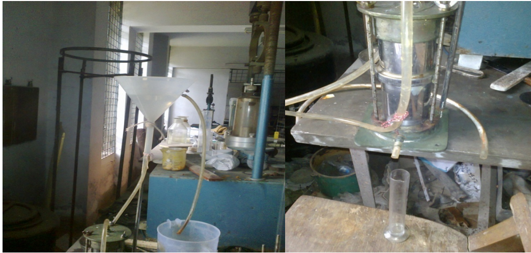
Figure 12: Constant head water permeability test of pervious concrete
