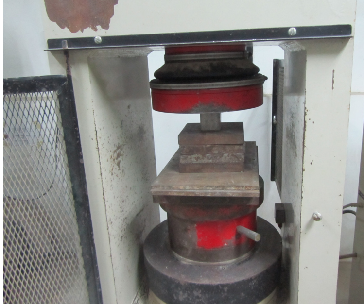
Figure 3 Picture of the compression machine used in determine compressive strength test of cube mortar specimens.
