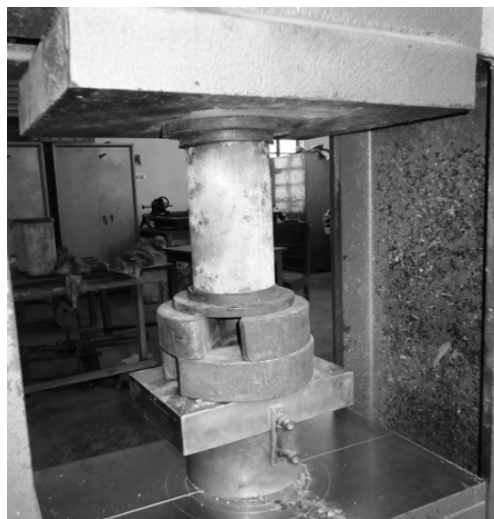
Figure 1: Test Set up for Compressive Strength of Concrete
