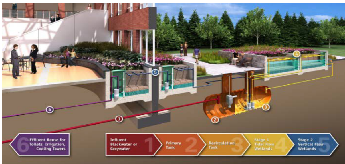
Figure- 3.1: Worrell's Living Machine—Constructed Wetlands in An Upscale Office Building
