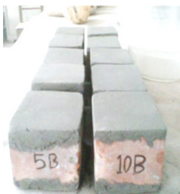
Figure 21: Typical mortar capping
