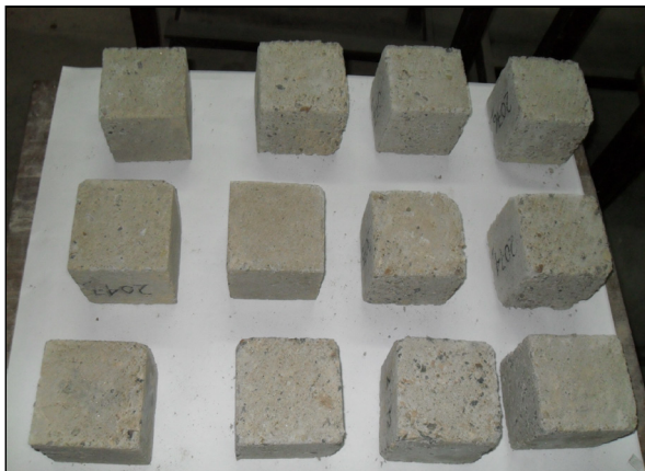
Plate No.2: FA Concrete specimens after 30 F-T cycles in PW
