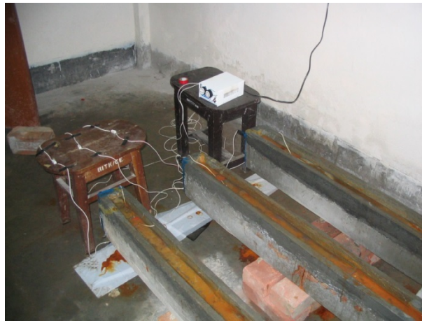
Figure 3: Test setup for accelerated corrosion
