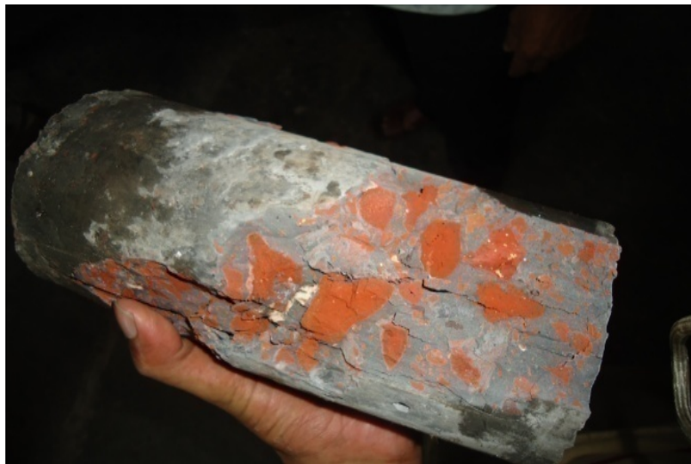
Figure 9: Failure behaviour of compressive strength test of pervious concrete
